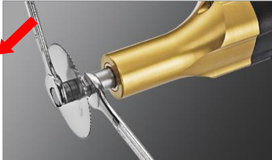
fig. 3 Releasing the retaining screw
